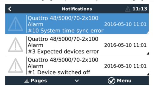
The real problem is Error 1. In this example it was caused by switching device L2 off with the front toggle switch. It was then quickly followed by Error 3. And when switching device L2 back on, briefly Error 10 is visible, followed by full recovery.
