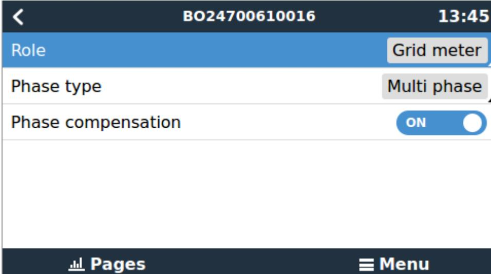
6. Make sure 'Role' is set to 'Grid meter', and 'Phase Type' matches your setup (i.e. single or multi phase).
