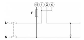
Note the jumper between terminals 1 and 4. You do not need this connection if you have the version AV2 of the sensor.
