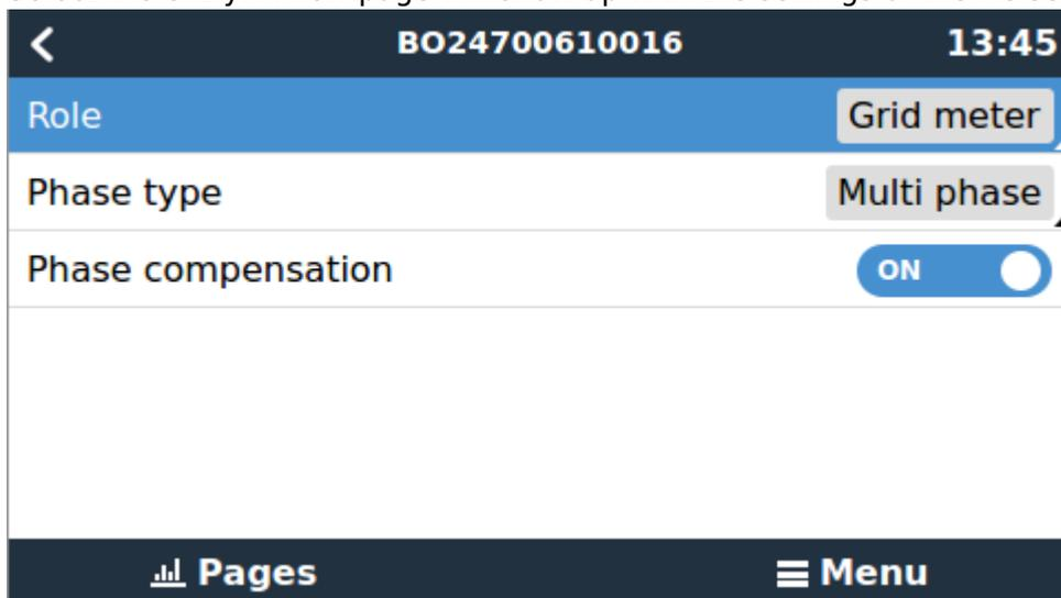
6. Make sure 'Role' is set to 'Grid meter', and 'Phase Type' matches your setup (i.e. single or multi phase).
