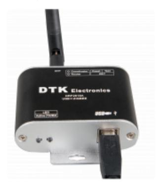
2. Connect the Zigbee to RS485 converter to the EM24 energy meter:
