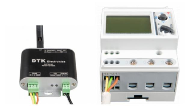
3. Make sure only one Zigbee device is powered up right now: the Zigbee to USB converter connected to the CCGX. Power down all others. *If you don't do this, the Zigbee to RS485 converter may be connected permanently to another Zigbee device.*
