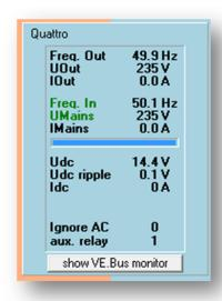
With Multi firmwares xxyy460 and up, VEConfig will indicate why the AC Input is rejected and will also show an indication of the remaining waiting time as a blue bar.
