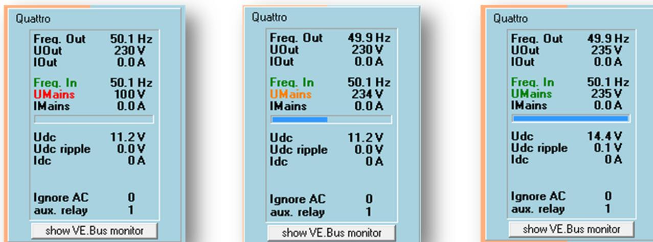
With Multi firmwares xxyy460 and up, VEConfig will indicate why the AC Input is rejected and will also show an indication of the remaining waiting time as a blue bar.
