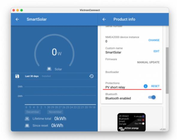
Note that the feature only shows when (a) the connected units features the protection, ie. 250/100 VE.Can model, HQ2150 and later; (b) requires the battery voltage to be between 10 and 15V; (c) requires VictronConnect v.580 or later; (d) requires firmware version v3.12 or later to be installed on the Solar Charger and (e) no error 80 to 83 is active.
