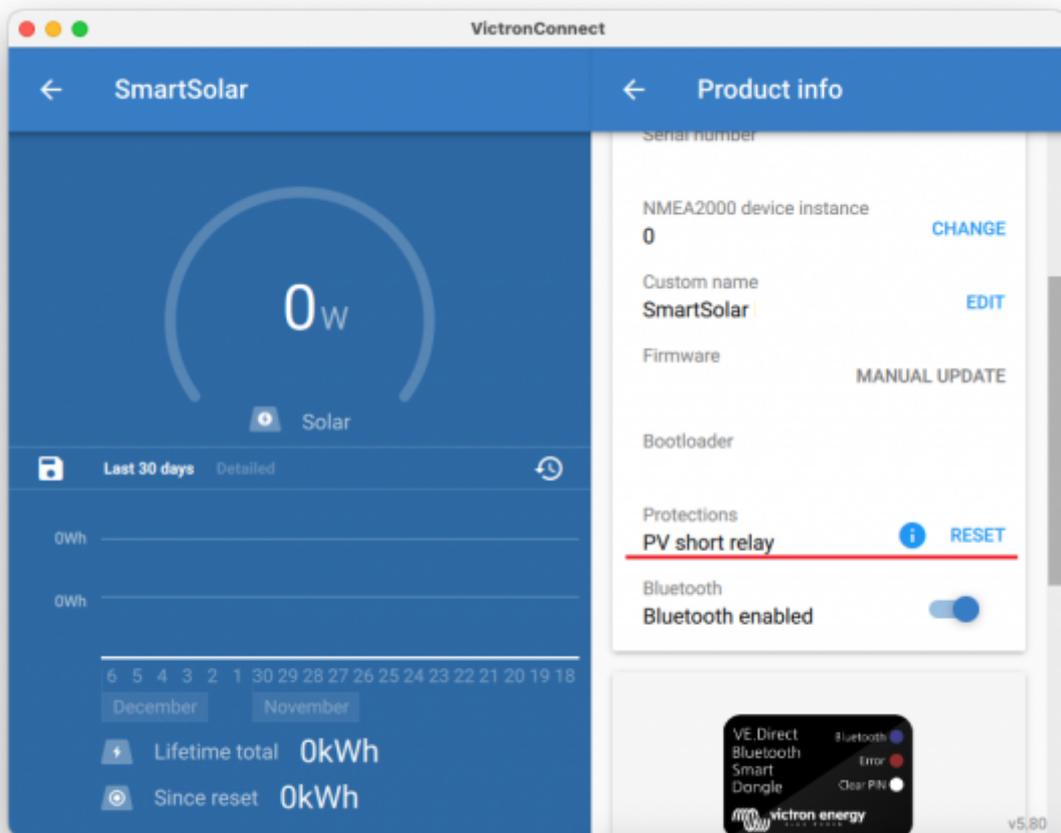
Note that the feature only shows when (a) the connected units features the protection, ie. 250/100 VE.Can model, HQ2150 and later; (b) requires the battery voltage to be between 10 and 15V; © requires VictronConnect v.580 or later and (d) requires firmware version v3.12 or later to be installed on the Solar Charger.
