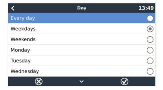
The Multi will start charging from the grid at the specified start time, and stop after the set duration or when the set SOC limit is reached. The period designated by the day, start time and duration will subsequently be referred to as a scheduled charge window.
