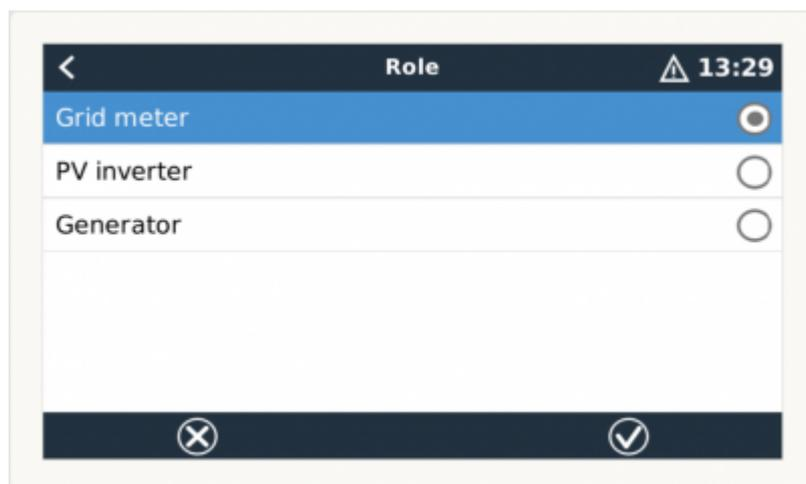
In GX device firmware version 2.80 and later - They can also be used for other purposes e.g. to measure specific, arbitrary AC loads or circuits for example. However it should not be considered a replacement to having a Victron inverter / charger. Attempting to use other brand battery inverters and trying to substitute their lack of data connectivity to the GX device by using energy meters will not work as expected.
