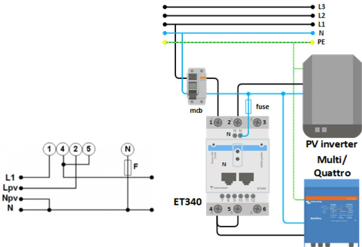
On the CCGX go to the grid meter in the Wired AC sensor settings. Make sure 'Phase type' is set to 'Single phase' and 'PV inverter on phase 2' is enabled.
