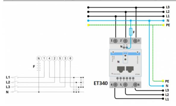
When used to measure a PV Inverter, terminals 1, 2 and 3 should face the PV inverter to ensure correct direction of current and power.
