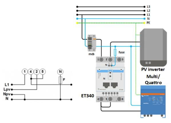
On the CCGX go to the grid meter in the Wired AC sensor settings. Make sure 'Phase type' is set to 'Single phase' and 'PV inverter on phase 2' is enabled.
