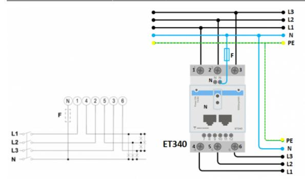
When used to measure a PV Inverter, terminals 1, 2 and 3 should face the PV inverter to ensure correct direction of current and power.
