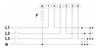
When used to measure a PV Inverter, terminals 1, 2 and 3 should face the PV inverter to ensure correct direction of current and power.
