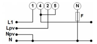
On the CCGX go to the grid meter in the Wired AC sensor settings. Make sure 'Phase type' is set to 'Single phase' and 'PV inverter on phase 2' is enabled.
