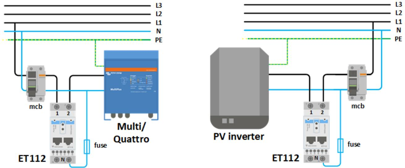
**Grid Meter** - Wiring when used as a grid meter. **PV Inverter** - Wiring when used to measure PV inverter or AC Genset.
