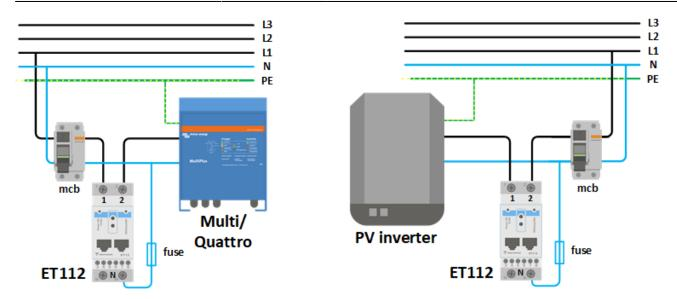
Wiring when used as a grid meter. Wiring when used to measure PV inverter or AC Genset.
