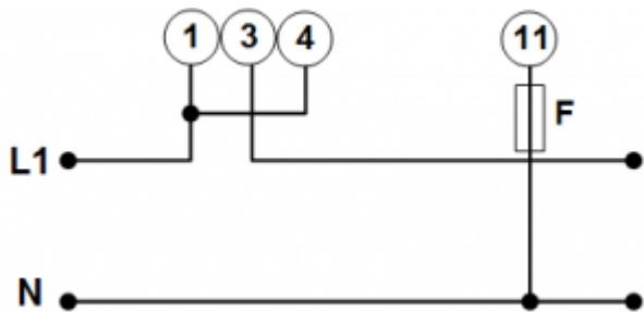
The diagram shows the wiring when used as a grid meter.
