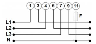
When used to measure a PV Inverter, terminals 1, 4 and 7 should face the PV inverter to ensure correct direction of current and power.
