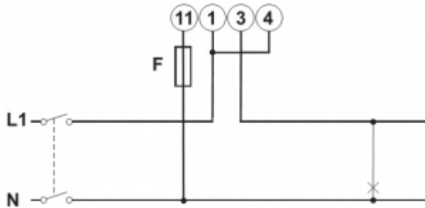
Note the jumper between terminals 1 and 4. You do not need this connection if you have the version AV2 of the sensor.
