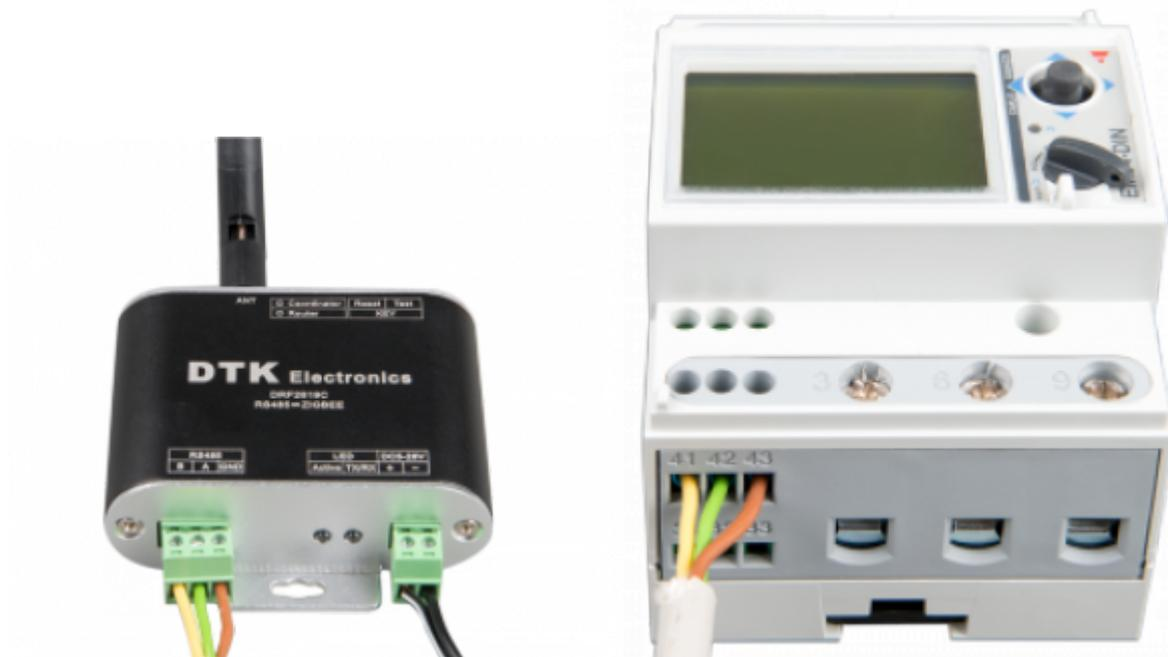
3. Make sure only one Zigbee device is powered up right now: the Zigbee to USB converter connected to the CCGX. Power down all others. *If you don't do this, the Zigbee to RS485 converter may be connected permanently to another Zigbee device.*
