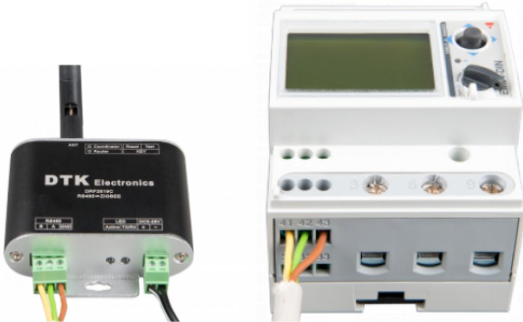
3. Make sure only one Zigbee device is powered up right now: the Zigbee to USB converter connected to the CCGX. Power down all others. *If you don't do this, the Zigbee to RS485 converter may be connected permanently to another Zigbee device.*
