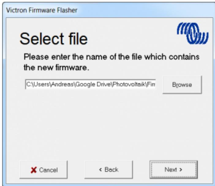
Last chance to disconnect 230VAC from the ECOmulti input. The VE.Bus cable of the CCGX must also be disconnected. Click "Next":
