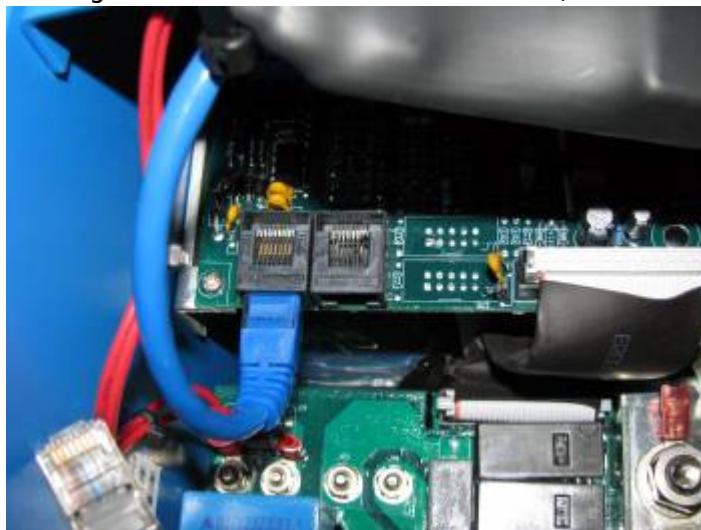
Cabling for MK2USB connected to ECOmulti (grey cable):
