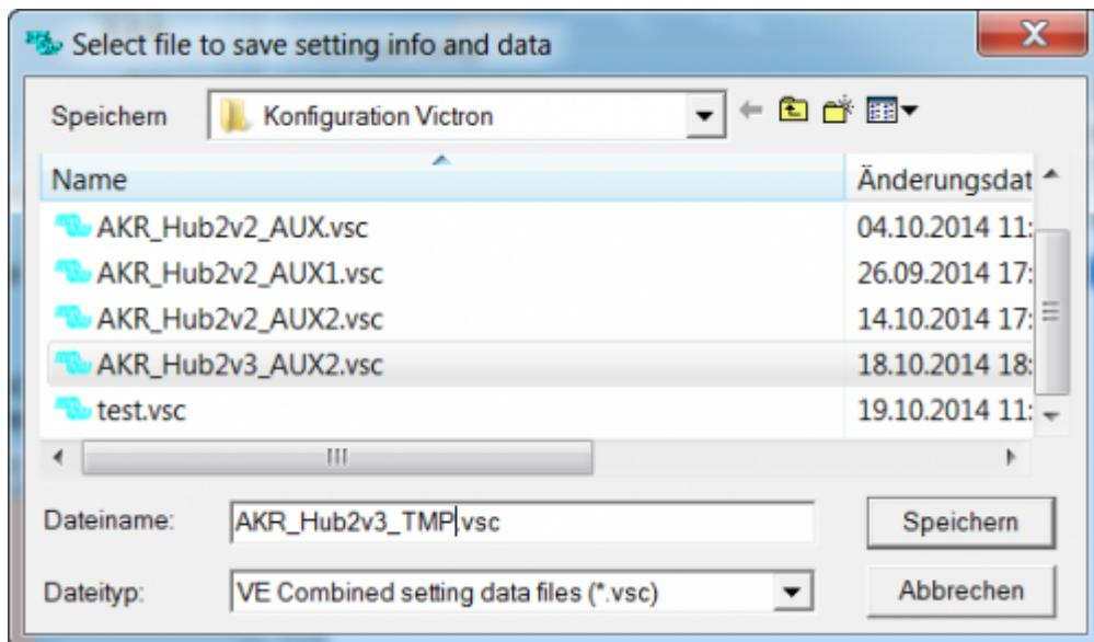
Use a meaningful filename. In this case the system name "AKR", The hub type "Hub2" and the input for the AC Sensor "TMP" are used. After clicking "Save" the the settings will be saved in a small file.
