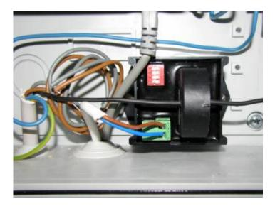
In the above image an installation cable  $2 \times 0.75 \text{mm}^2$  is used for connecting the sensor to the ECOmulti. Tests have shown, that a shielded cable doesn't improve the values. An installation cable is enough. The brown wire is plus, the blue wire is minus!
