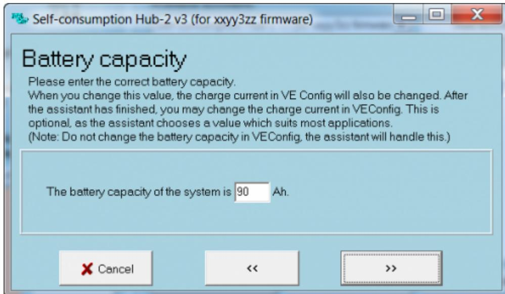
Check battery capacity. It should be 90Ah for the LiFePo4 batteries. Click "»":
