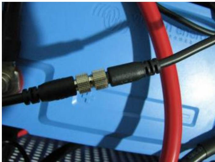
Connect the BMS cables to the VE.Bus BMS in the ECOMulti:
