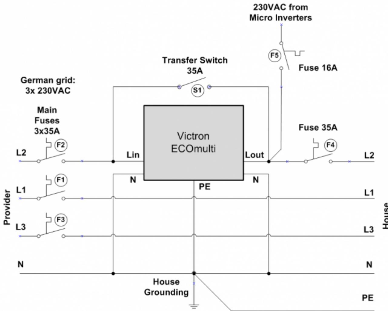
The photovoltaic energy (in this case 230VAC/12A from micro inverters) will be fed into the house L2 phase on the output of the ECOmulti (=Hub2). An extra fuse F5/16A is protecting the solar system.
