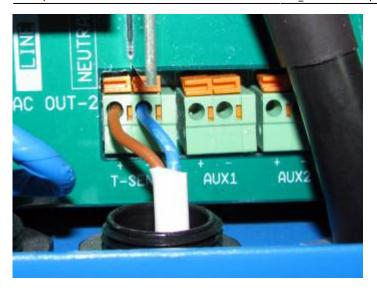
The cable leads to the T-Sense input of the ECOmulti: plus on the left (brown) and minus on the right side (blue). AUX1 and AUX2 can only be used on the newest ECOmultis, the recommendation is to use the T-Sense input. This will work on all ECOmultis.
