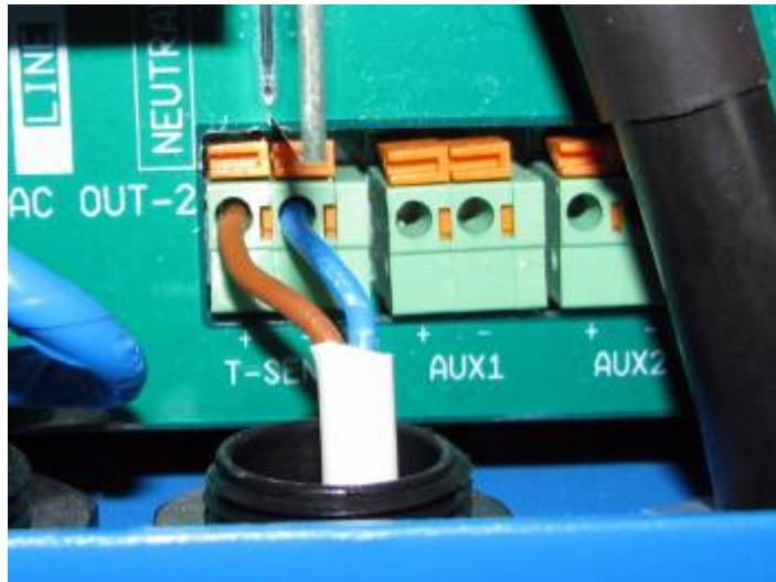
The cable leads to the T-Sense input of the ECOmulti: plus on the left (brown) and minus on the right side (blue). AUX1 and AUX2 can only be used on the newest ECOmultis, the recommendation is to use the T-Sense input. This will work on all ECOmultis.
