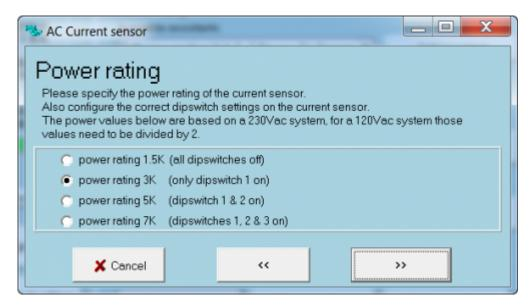
For a Hub2 system, the photovoltaic output must be connected to the ECOmulti output. Select the middle option and click ">":
