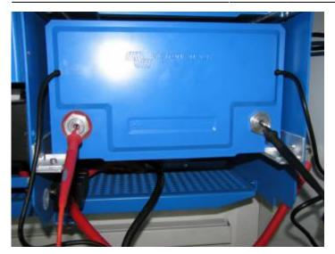
• Each of the batteries should have about 13.3VDC:
