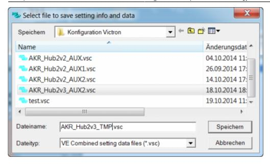
Use a meaningful filename. In this case the system name "AKR", The hub type "Hub2" and the input for the AC Sensor "TMP" are used. After clicking "Save" the the settings will be saved in a small file.
