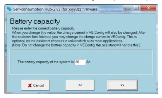
Check battery capacity. It should be 90Ah for the LiFePo4 batteries. Click "»":
