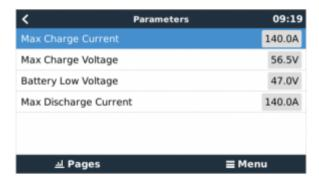
This parameters page is also a good place to check that all batteries are connected and working properly. In normal working conditions, the current limit is 25A per cell. For example, 100A charge current limit (100 / 25 = 4) means there are 4 Pylontech battery modules connected.
