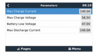
This parameters page is also a good place to check that all batteries are connected and working properly. In normal working conditions, the current limit is 25A per cell. For example, 100A charge current limit ( 100 / 25 = 4 ) means there are 4 Pylontech battery modules connected.
