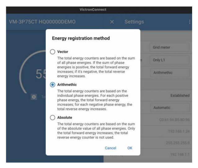
**Phase Compensation (Sum/Vector Method):** It is common for 3 phase grid utility meters calculate energy by summing all phases. If your meter does this, VRM (Victron Remote Management) should also show this summed (compensated) energy, or else there will be a discrepancy.
