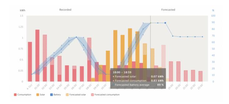
On the left side of the vertical line, you see the recorded values. On the right side of the line it shows the solar forecast, the consumption forecast and also the target SOC that will be followed (as scheduled during the last calculation for the site).
