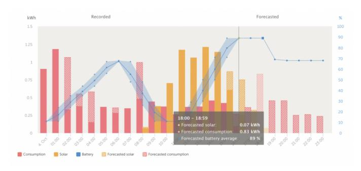
On the left side of the vertical line, you see the recorded values. On the right side of the line it shows the solar forecast, the consumption forecast and also the target SOC that will be followed (as scheduled during the last calculation for the site).
