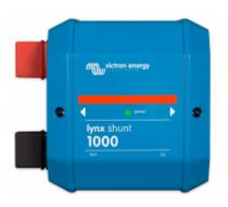
The Lynx shunt contains a positive bus-bar with space to mount a fuse and a negative bus-bar with a shunt. It also contains battery monitoring electronics. The Lynx shunt can send via the VE.CAN bus battery monitoring information to a CCGX or VGX or to a third party CANbus monitoring system, such as a NMEA2000. The CCGX, VGX or third party display acts as battery monitor display and is also used to set up the built-in battery monitor.
