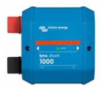
The Lynx shunt contains a positive bus-bar with space to mount a fuse and a negative bus-bar with a shunt. It also contains battery monitor electronics. The Lynx shunt can send via the VE.CAN bus battery motoring information to a CCGX or VGX or to a third party can bus monitoring system, such as a NMEA2000 (check with Johannes). The CCGX, VGX or third party display acts as battery monitor display and is also used to set up the built-in batter monitor.
