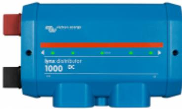
Contains positive and negative bus-bar and provides a connection for for 4 individual DC equipment or load or DC groups. It has a space for a individual DC fuses per DC group and a led for each fuse to indicate if fuse is blown.
