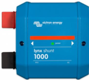
The Lynx shunt contains a positive bus-bar with space to mount a fuse and a negative bus-bar with a shunt. It also contains battery monitor electronics. The Lynx shunt can send via the VE.CAN bus battery monitoring information to a CCGX or VGX or to a third party can bus monitoring system, such as a NMEA2000 (check with Johannes). The CCGX, VGX or third party display acts as battery monitor display and is also used to set up the built-in batter monitor.
