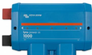
The lynx power in module is used to connect batteries. It contains a negative and positive DC bus-bar with M8 bolts to connect batteries cables to.
