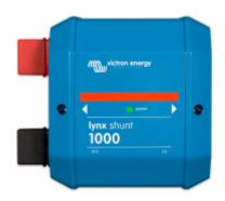
The Lynx shunt contains a positive bus-bar with space to mount a fuse and a negative bus-bar with a shunt. It also contains battery monitor electronics. The Lynx shunt can send via the VE.CAN bus battery motoring information to a CCGX or VGX or to a third party can bus monitoring system, such as a NMEA2000 (check with Johannes). The CCGX, VGX or third party display acts as battery monitor display and is also used to set up the built-in batter monitor.
