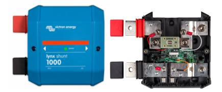
The Lynx shunt contains a positive bus-bar with space to mount a CNN fuse and a negative bus-bar with a shunt. It also contains battery monitoring electronics. The Lynx shunt can send via the VE.CAN bus battery monitoring information to a GX device (Cerbo GX) or to a third party CANbus monitoring system, such as a NMEA2000. The GX device (Cerbo GX) or third party display acts as battery monitor display and is also used to set up the built-in battery monitor.
