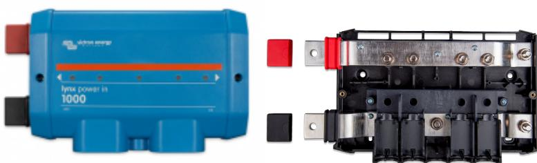
The lynx power in module is used to connect batteries via an external fuse. It can be useful if you have multiple parallel strings. Due to the extremely high short circuit current potential of most battery banks, it is suggested to use an external fuse system with an appropriate fault current interruption rating (such as an NH HRC).
