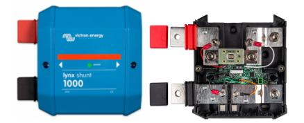
The Lynx shunt contains a positive bus-bar with space to mount a CNN fuse and a negative bus-bar with a shunt. It also contains battery monitoring electronics. The Lynx shunt can send via the VE.CAN bus battery monitoring information to a CCGX or VGX or to a third party CANbus monitoring system, such as a NMEA2000. The CCGX, VGX or third party display acts as battery monitor display and is also used to set up the built-in battery monitor.
