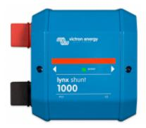
The Lynx shunt contains a positive bus-bar with space to mount a CNN fuse and a negative bus-bar with a shunt. It also contains battery monitoring electronics. The Lynx shunt can send via the VE.CAN bus battery monitoring information to a CCGX or VGX or to a third party CANbus monitoring system, such as a NMEA2000. The CCGX, VGX or third party display acts as battery monitor display and is also used to set up the built-in battery monitor.
