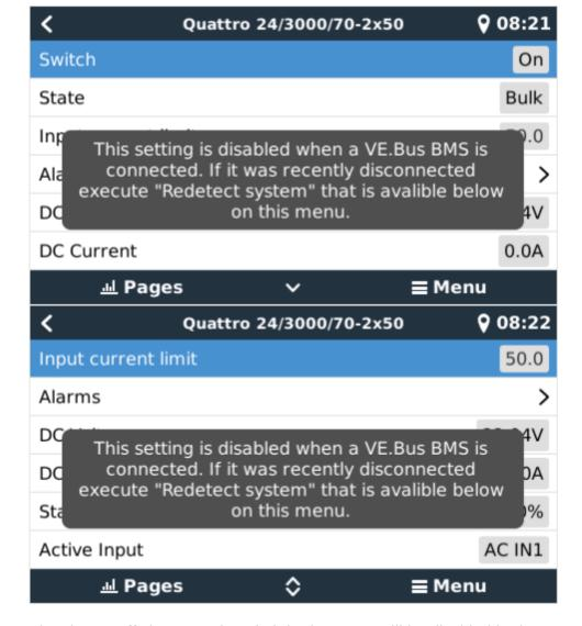
Also the *on/off/charger only* switch in the CCGX will be disabled in the case.
