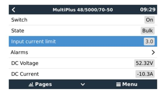
The limit as set by the user in the CCGX will be applied to all inputs where 'Overruled by remote', configured with VEConfigure, is enabled:
