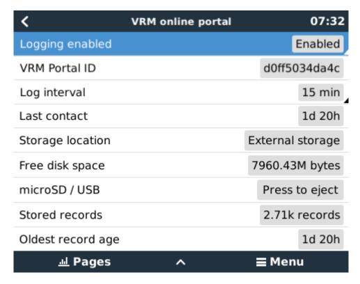
When using this external memory, it will still make use of an active internet connection to send its backlog. That means that even with months worth of backlog, once the CCGX re-acquires an Internet connection, all of the backlog is sent out. And because of an enhanced algorithm, this takes considerably less time and traffic than before.
