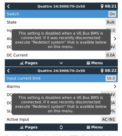
Also the *on/off/charger only* switch in the CCGX will be disabled in the case.
