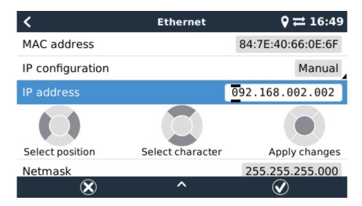
Complete details of IP requirements, as well as used port numbers will be found in the VRM FAQ - ports and connections used by the CCGX.
