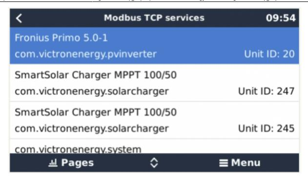
Additionally this information is also documented on the 'Unit ID mapping' tab in the Modbus-TCP excel sheet.
