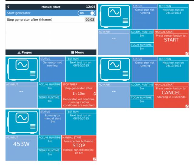
**WARNING:** If the generator is started manually (remotely) without using the stop timer, it will run until the 'Off' button has also been manually toggled.
