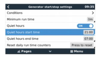
Quiet hours allows you to define a period during which the noise from a running generator would be a
