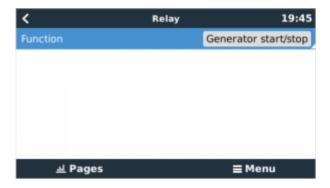
Now that has been enabled, all the settings pertaining to the *Automatic Generator Start/Stop* function will be found in the main Menu under: Settings → Generator start and stop.
