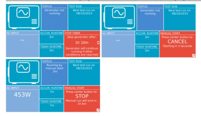
**WARNING:** If the generator is started manually (remotely) without using the stop timer, it will run until the 'Off' button has also been manually toggled.
