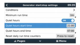
Quiet hours allows you to define a period during which the noise from a running generator would be a nuisance; and to set different values to the conditions which would cause an auto-start during this period - thus ensuring that the generator will only start during a quiet period when it is absolutely necessary.
