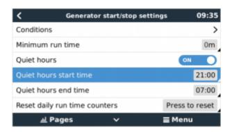
Quiet hours allows you to define a period during which the noise from a running generator would be a nuisance; and to set different values to the conditions which would cause an auto-start during this period - thus ensuring that the generator will only start during a quiet period when it is absolutely necessary.
