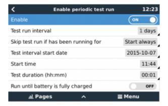
• **Test run interval**: Set the interval between test runs.
