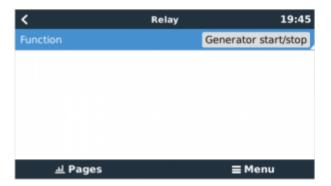
Now that has been enabled, all the settings pertaining to the *Automatic Generator Start/Stop* function will be found in the main Menu under: Settings → Generator start and stop.
