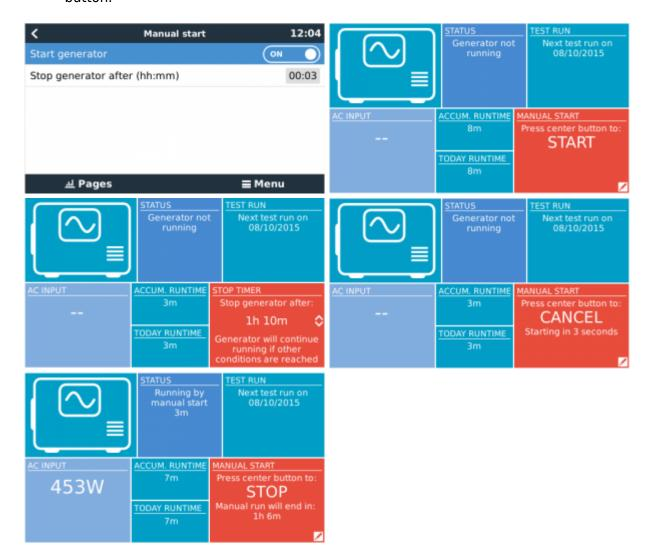
**WARNING:** If the generator is started manually (remotely) without using the stop timer, it will run until the 'Off' button has also been manually toggled by the user.
