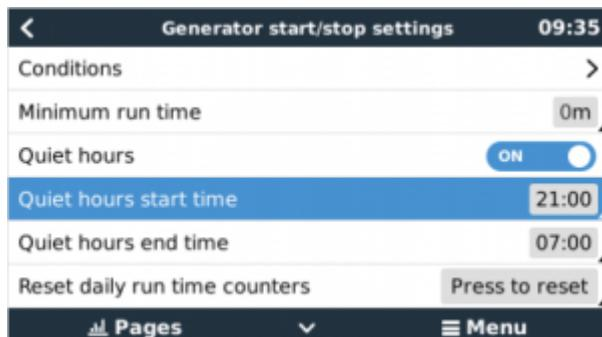
Quiet hours allows you to set a time zone for nighttime with values that make the generator start only when is really necessary.
