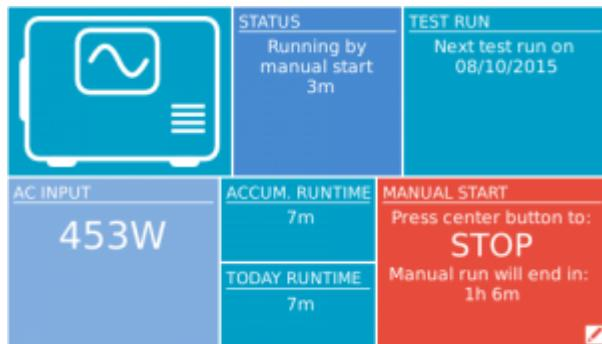
**WARNING:** If the generator is started manually (remotely) without using the stop timer, it will run until the 'Off' button has also been manually toggled by the user.
