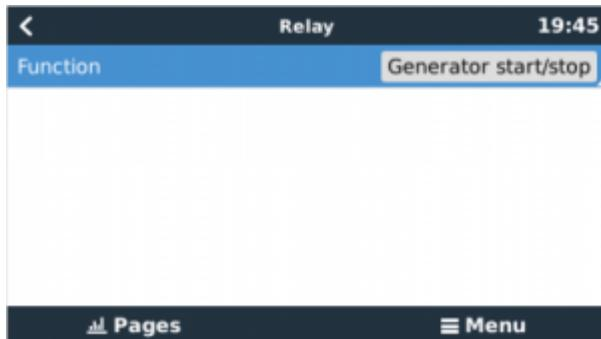
Go to: Settings → Relay and set *Function* to "Generator start/stop"
