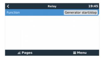
Go to: Setttings → Relay and set *Function* to "Generator start/stop"
