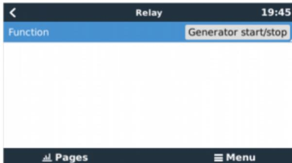
Go to: Settings → Relay and set *Function* to "Generator start/stop"
