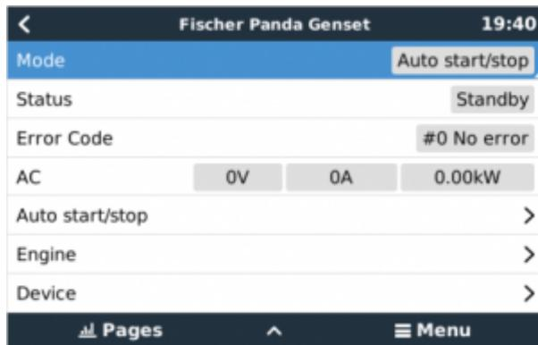
1. Enable the "AutoStart" function in the Fischer Panda generator control panel.
