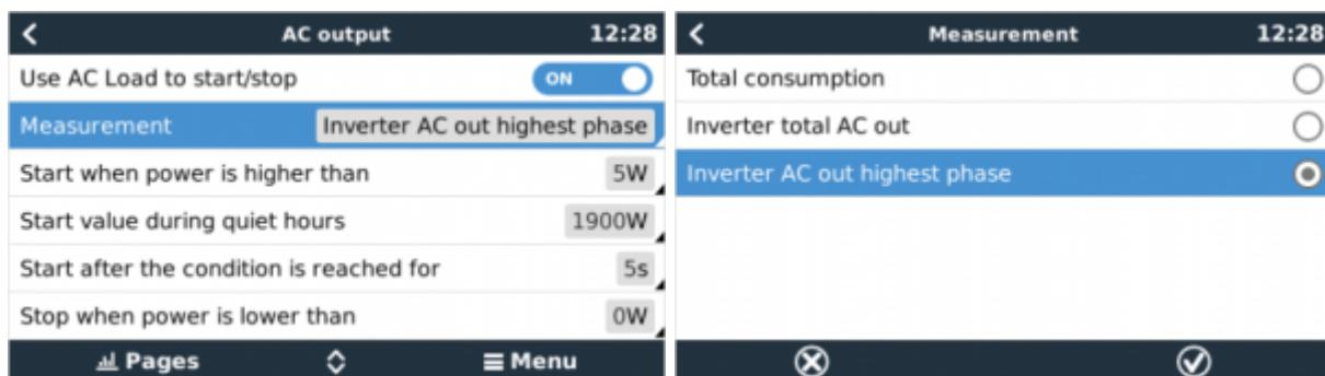
The “Measurement” setting is available on firmware v2.0 and onwards and has three possible values:
