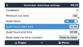
Quiet hours allows you to set a time zone for nighttime with values that make the generator start only when is really necessary.
