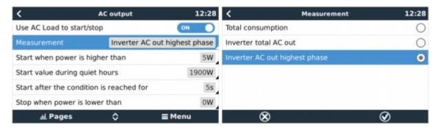
The "Measurement" setting is available on firmware v2.0 and onwards and has three possible values:
