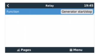
Go to: Setttings  $\rightarrow$  Relay and set function to "Generator start/stop"
