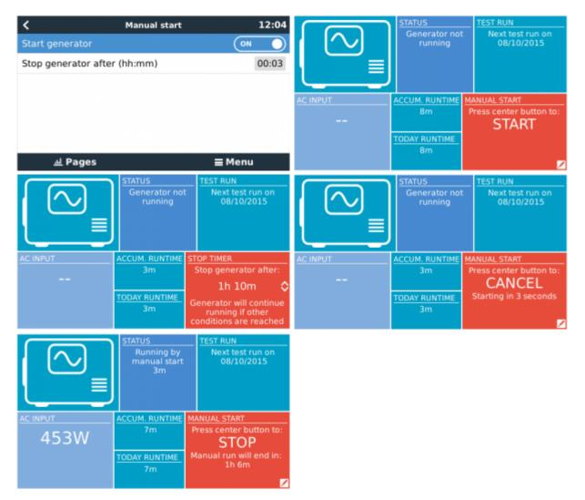
**WARNING:** If the generator is manually started without a stop timer, won't stop until the user set to off the manual start option.
