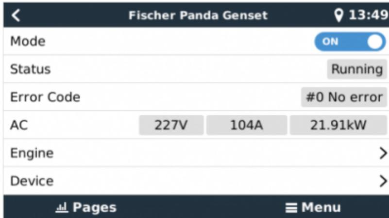
Notice that it features an on/off switch as well as displaying status information, and the main AC parameters: voltage, current and power.
