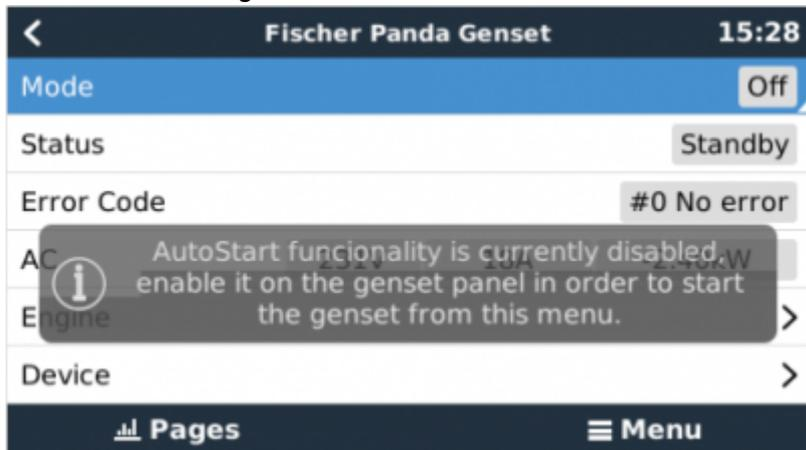
If the generator auto start/stop is enabled, it will show error #1 Remote switch control
