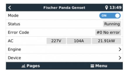
Notice that it features an on/off switch as well as displaying status information, and the main AC parameters: voltage, current and power.
